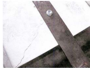
FIG.3 200MM EDGE DISTANCE CONCRETE RUPTURE
