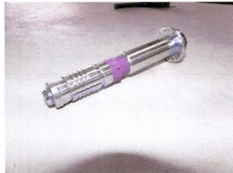
FIG.1 BRACE PANEL BOLT
